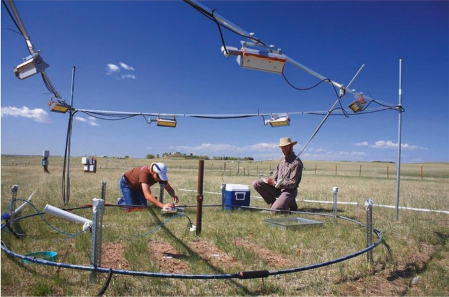
**Fig. 4.6** The Prairie Heating and CO<sub>2</sub> Enrichment (PHACE) study located manipulated temperature and CO<sub>2</sub> concentration in C3–C4 shortgrass steppe. Warming was controlled by infrared heaters at the top of each plot, while CO<sub>2</sub> was controlled by emitting gas from the ring at the bottom of the plot (photograph by Sam Cox, (former) USDA-ARS Biological Science Technician, (now) Natural Resource Specialist with Wyoming BLM)
